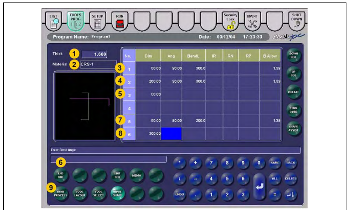
Abb. 7-68 „INPUT SHAPE“-Display (SHAPE-Modus)
