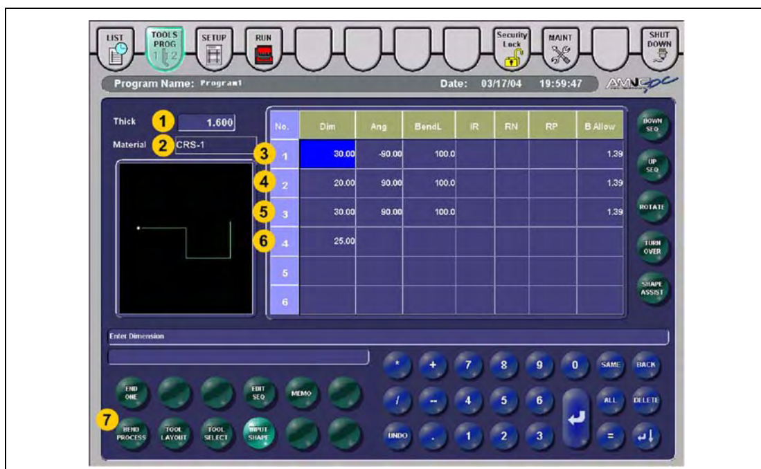
Abb. 7-79 „INPUT SHAPE“-Display (SHAPE-Modus)
